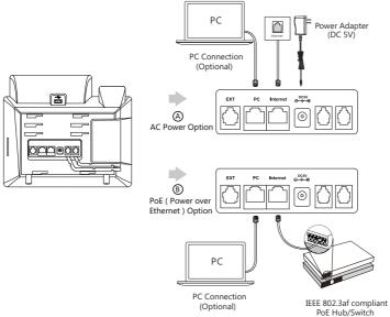
Note: The IP phone should be used with Absolute VOICE original power adapter (5V/2A) only. The use of the third-party power adapter may cause the damage to the phone. If you are connecting a PC to your phone, we recommend that you use the Ethernet cable provided by Absolute Communications. If inline power (PoE) is provided, you don't need to connect the power adapter. Make sure the hub/switch is PoE-compliant.
