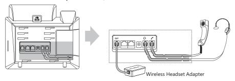
Note: The headset or wireless headset adapter EHS36/EHS40 should be purchased separately. The EXT port can also be used to connect the expansion module EXP40. For more information on how to use the EHS36, EHS40 and EXP40, refer to Yealink EHS36 User Guide, Yealink EHS40 User Guide and Yealink EXP40 User Guide.
